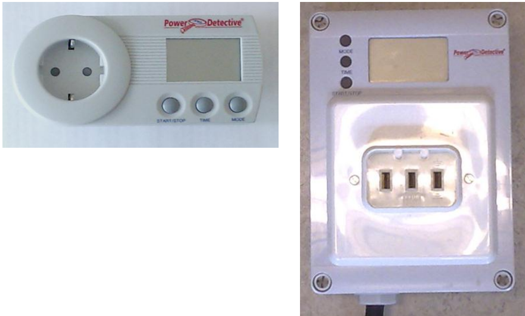
Figure 2 Power Detective - plugs for metering of end-use demand. The rightmost picture shows metering of the demand for an electric cooker [9]
