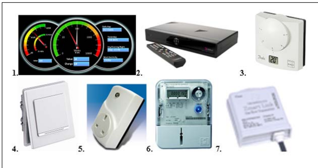
Figure 1: SMaRT Action System Components; 1. Energy Speedo Display, 2. 3View Set-Top-Box, 3. Room Thermostat, 4. Light Switch, 5. Appliance Plug, 6. Electricity Meter, 7. Gas Meter Logger.
