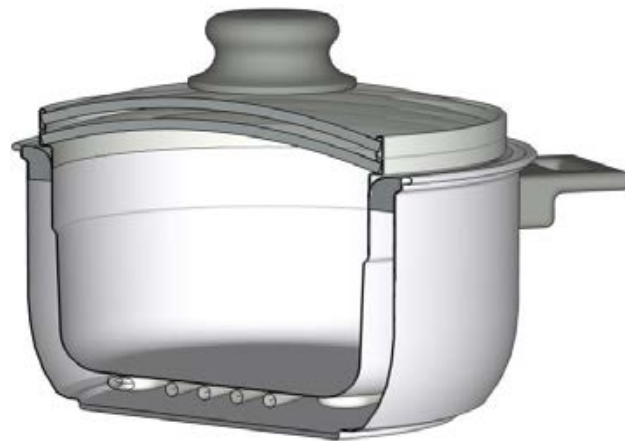
Figure 1. Section view of EffiCooker
