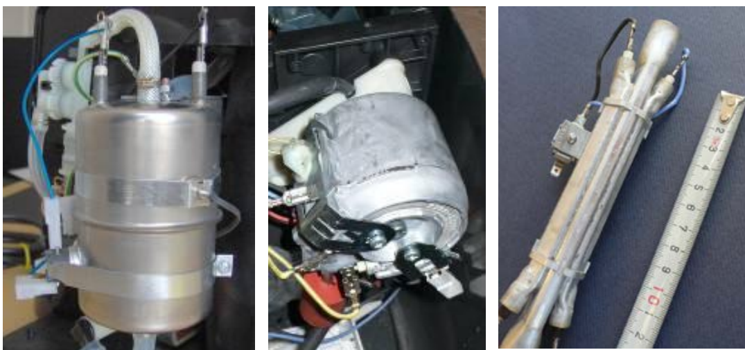
Figure 2. Heating units of coffee machines: Boiler (left), thermo-block (middle) and flow-type heater (right). Source: Topten
