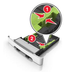
Note: Use the paper size indicators on the bottom of the tray to help position the guides.
