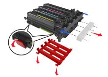
**Warning—Potential Damage:** Do not touch the shiny photoconductor drum under the imaging kit. Doing so may affect the quality of future print jobs.
