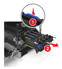
8 Remove the used developer unit.
