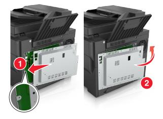
6 Turn the screws clockwise to lock the cover.
