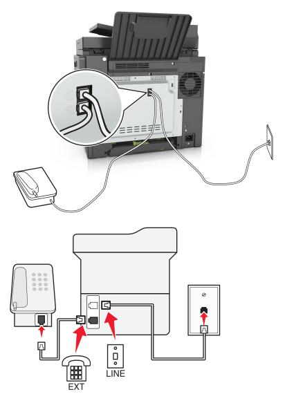
Setup 2: Printer is connected to a wall jack; cable modem is installed elsewhere in the facility
