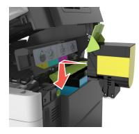
**5** Slide and hold the release latch on the right side of the printer, and then slowly close the top door.
