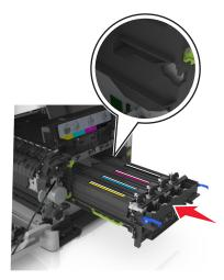
Gently but firmly push the blue levers down until the imaging kit fits into place.
