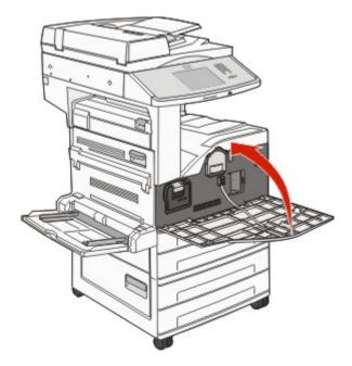
**Note:** After you insert the photoconductor and close all the doors, the printer performs a motor cycle and clears the Replace Photoconductor warnings.
