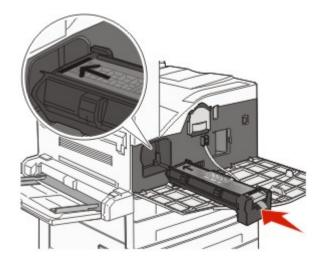
Remove the tape from the top of the photoconductor.
