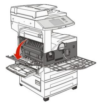
Pull the photoconductor out of the printer.
