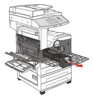
Place the photoconductor on a flat, clean surface.
