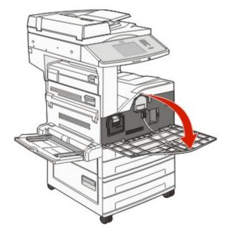
**Note:** The photoconductor cannot be pulled out if Side Door A is closed.
