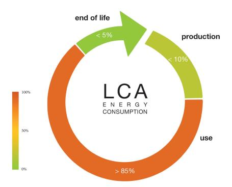
Fig 2.7: Simplified LCA for the energy consumption of a refrigerator during irs life time.
