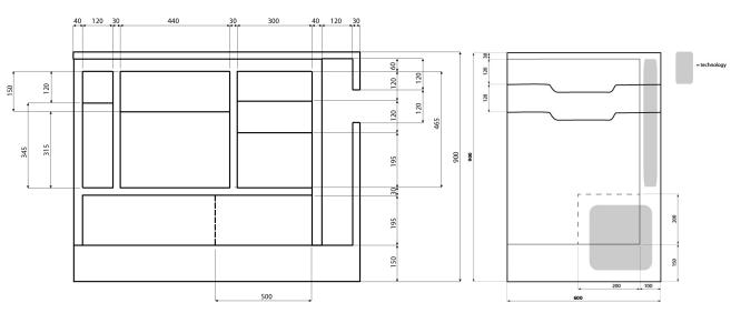
Fig. 9.43: Dimensions of all the compartments of Pompador.
