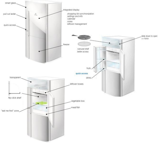
Fig.8.4-6: The Organized, closed and opened with its compartments and features indicated. Inside the top compartment with slide-down-to-open smart glass door, there is carusel shelf. The pull-out larder on the side is for quick access to fruits and drinks. In the large compartment there is an "eat-me-first zone" and a system for post-prepared food.
