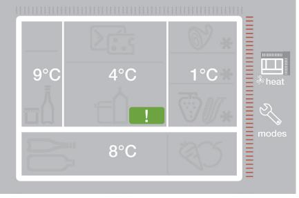
Fig. 9.38: The EatSoonZone is marked in the display if it is well loaded. The "!" denotes there is a notification for someone about something that has to be eaten. The red Idashed lines on the sides of the refrigerator icon indicates where the warm air is directed and it can be swithced by pressing on it.
