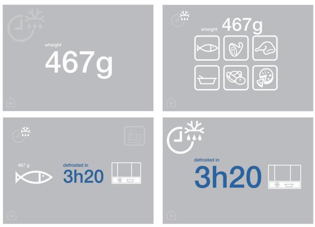
Fig. 9.30: The interface for thawing. When frozen food is placed on the scale its wheight is first shown.
