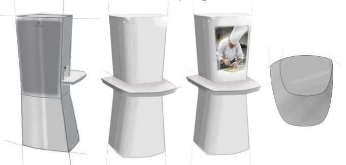
Fig. 8.17-20: The front view with a large integrated display on the door and a water tap to the right. The back view with a table and. The display and and cocking instructions from a virtual chef can be visible on the backside too. 18. The top view.
