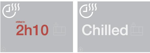
Fig 9.28: The interface for chilling food. When hot food is placed on the top surface the display shows the time it will take before it is chilled enough to be placed in the refrigerator.
