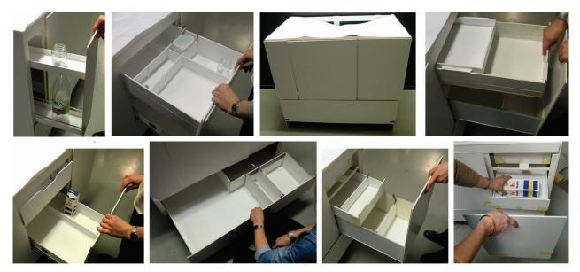
Fig 8.23: The paper mock-up from different views. All the interior parts were built to try dimensions and handling.
