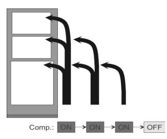
Fig 8.24 Schematic picture over how the distrubution of cold air can work with dampers if there are three compartments/zones with different temperatures.
