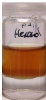
Figure 4.10 Lignin (0.5 g/L) dissolved in an aqueous-organic two-phase system consisting of NaAc buffer (0.1 M, pH 4.5) and 1-hexanol. At non-saturating concentrations ( < 1 g/L) no crud layer at the interphase was formed.
