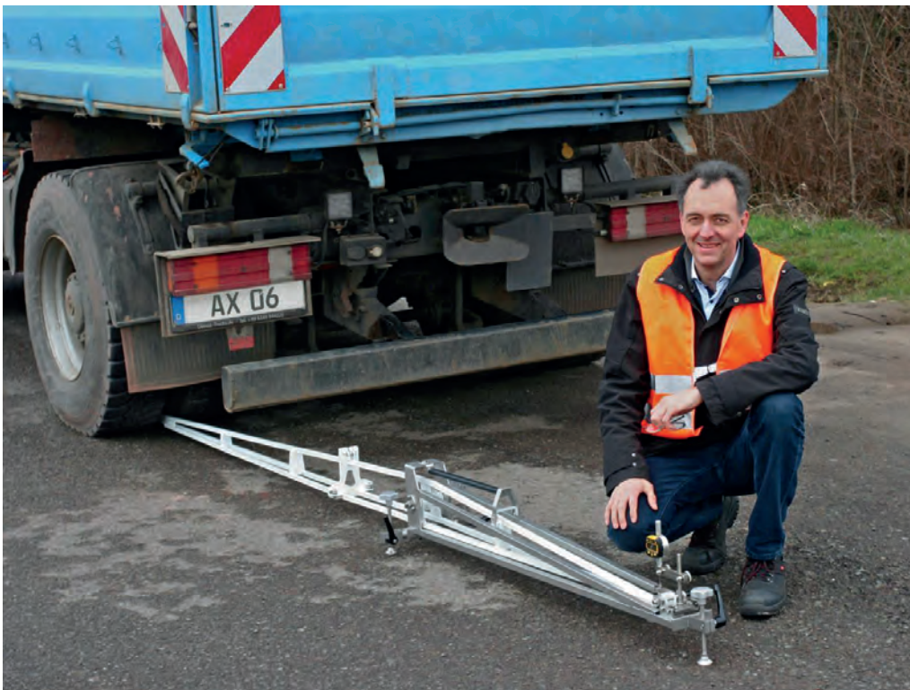
Figure 7. The classical Benkelman beam AX06 with a dial gauge
