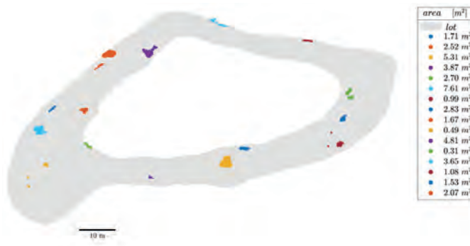
Figure 6. Identified weak spot clusters within the inspection lot in Fig. 3 based on the FCM method.
