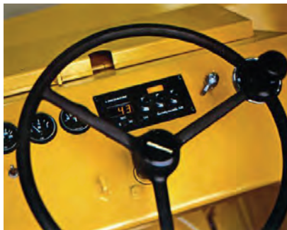
Figure 1. Early Compactometer installed in a roller.
