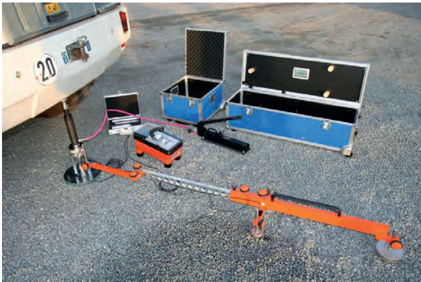
Figure 1. Set up of the static plate load test device AX01a
