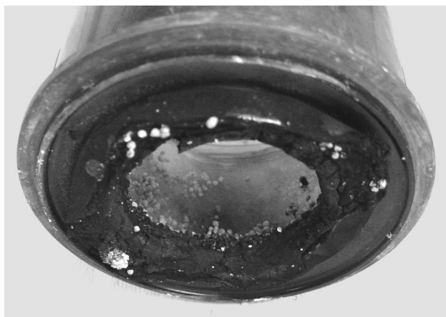
Fig. 2. Base of the upper absorbent canister from the absorber assembly in which the fire occurred, showing melting and deformation of the canister seal and the carbon dioxide absorbent cartridge.
