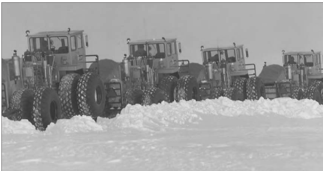
ABOVE—Winterized surveyor and shothole drilling rig on Alaska's North Slope (1960s). BELOW—Seismic vibrators working under the same winter conditions but a decade later. (courtesy Western Geophysical Company).
