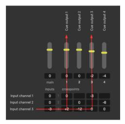
These images show a close-up view of the **cue matrix mixer** in QLab (with some additional annotations). The top row, row 0, contains the output level controls. Each successive row represents an input with audio entering the mixer on the left edge and flowing to the right.
