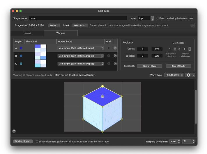
Imagine the output route is connected to a projector that is pointing at a cube-shaped object on stage. Here, the three regions are each warped to conform to a single face of the cube, and the control points on each region that coincide with controls points on other regions are linked. This allows you to warp the regions to fit the cube as a single object, instead of three separate objects.
