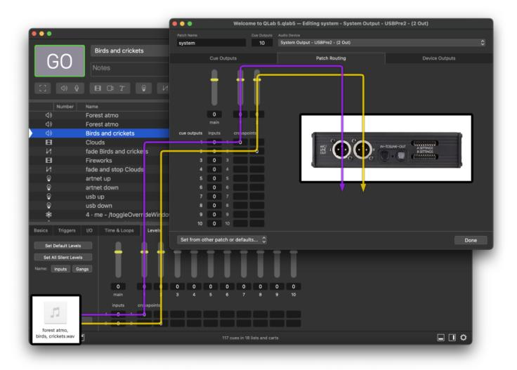
In this example, the file target of the cue named "Birds and crickets" is a two-channel wav file named forest atmo, birds, crickets.wav. The audio from the first channel of this audio file is represented by the purple arrow, and the second channel is represented by the yellow arrow.
