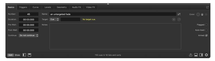
Because prices Fade cues can target both cues and patches, a pop-up menu appears next to the Target field to switch between cue targeting and patch targeting. When *Patch* is selected from this menu, a second pop-up menu appears which allows you to select the patch that you want to fade.
