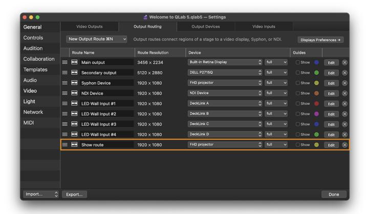
The result is that every pixel of the device is utilized to display every pixel of the cue. Since the stage, route, and device all have a resolution of 1920 × 1080, there is a straight one-to-one correspondence between the cue's pixels and the device's pixels.
