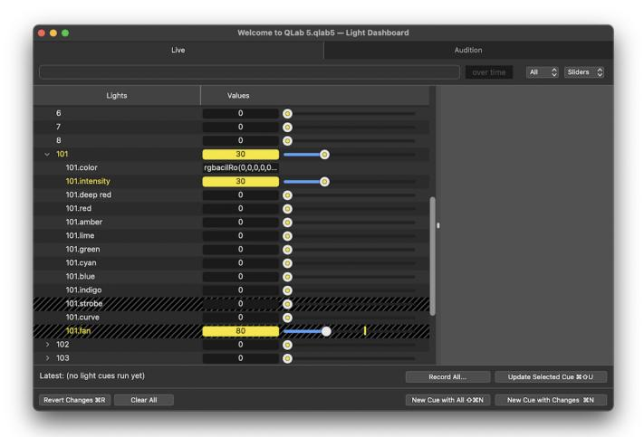
In this screen shot, two parameters of the light called 101 have been parked: the strobe parameter is parked at 0, and the fan parameter is parked at 160. The fan parameter has subsequently been set to 80, and the light mark shows that the current live value of the fan parameter remains at 16. All other parameters of the instrument remain unparked and can be used as normal.
