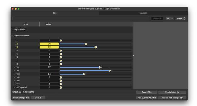
Here, a P Light cue has been run which raised instrument 4 to 24 and instrument src4 to 69. Then, instrument 2 has been manually set to 36 and instrument 3 has been manually set to 50
