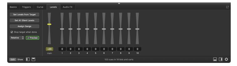
In this screen shot, the  $\{+\}$  Fade cue raises the main level of its target cue by 20 db. So if the main level of target cue were set at -40, running this  $\{+\}$  Fade cue would bring the main level to -20. If the main level of the target cue were set at -10, running this  $\{+\}$  Fade cue would bring the main level to +10.
