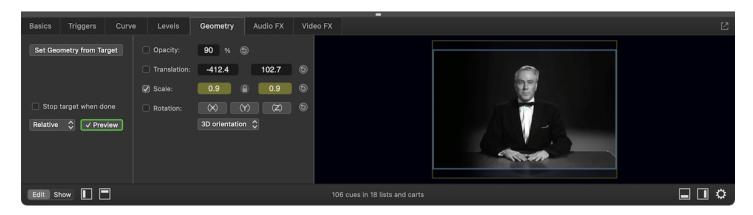
In this screen shot, the  $\{\cdot\}$  Fade cue has its scale set to 0.9 which has the effect of reducing the size of the target to 90 % of its current size. If you ran the  $\{\cdot\}$  Fade cue three times, the cumulative result would be reducing the size of the target cue to 72.9 % of its original size, since each time the  $\{\cdot\}$  Fade cue runs, it causes a 90 % reduction of the then-current size.
