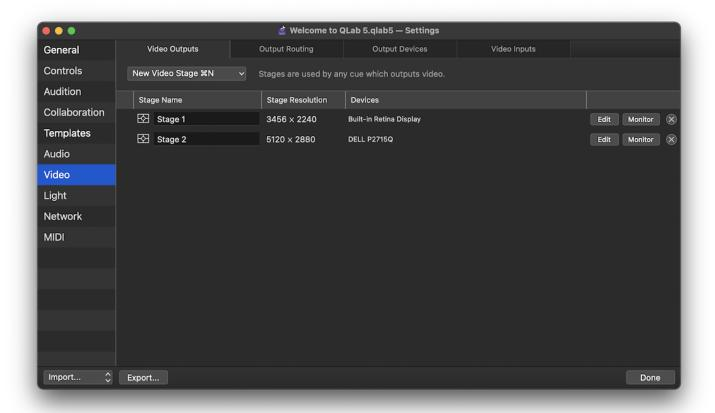
This screen shot was taken on a 2021 16" MacBook Pro with a 5120 × 2880 monitor connected to its HDMI port. When this workspace was created, QLab automatically created Stage 1 with the MacBook Pro's internal display assigned to it, and Stage 2 with the external monitor assigned to it.
