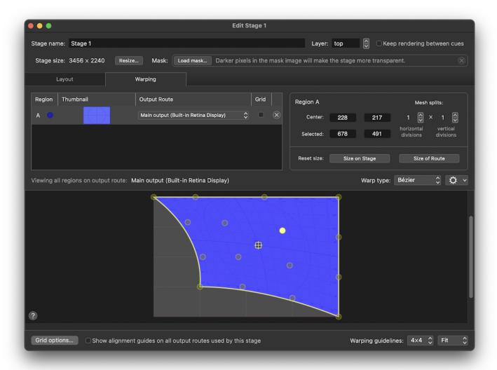
This warp type gives you sixteen control points per mesh split, and each control point bends the warp smoothly in the direction that it's pulled, as though the region is made of an elastic material.
