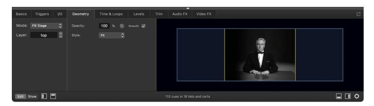
A cue using the **Fit** style will be symmetrically scaled as large as possible to display the entire image without changing the aspect ratio of the cue's file target. If the aspect ratio of the cue's file target is different than the aspect ratio of the stage, there will be blank space to the sides or above and below. QLab does not fill this space with black pixels; if there is a cue on a lower layer that truly fills the stage, it will be seen in these empty spaces.
