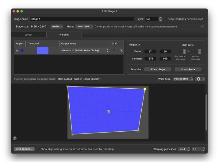
Using perspective warping, a projected object will appear the same size no matter where it's placed on the region. However, in order to allow complex perspective warped shapes, QLab uses "continuous perspective" warping which guarantees continuity of the warp, but means that extreme warps might not be truly 100% perspective-correct.
