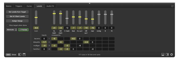
A key concept here is that if multiple 1/7 Fade cues share a target, but each 1/7 Fade cue has different active controls, then those 1/7 Fade cues can run simultaneously without interfering with each other. Because of this, in the scenario with a four-channel (1) Audio cue fading amongst seven speakers, very complex fades can be achieved by using simultaneous 1/7 Fade cues with different active controls, different curve shapes, and different durations.
