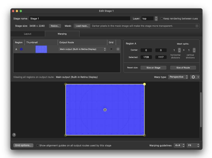
The purpose of the Warping Tab is to let you adjust the geometry of the stage on a per-region basis. Regions can be warped for any number of reasons, the most straightforward of which is to correct for keystoning caused by an off-axis projector. Warping can also be used to match a video projection to a non-flat projection surface, or for other creative effects.
