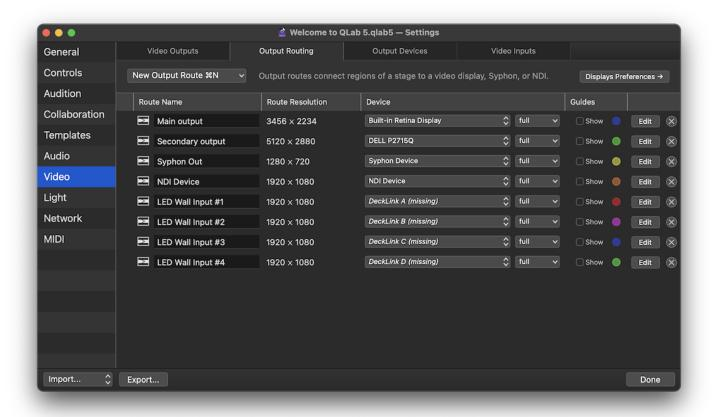
This workspace contains eight output routes of various types. The output routes in the workspace are listed in a table with several columns.
