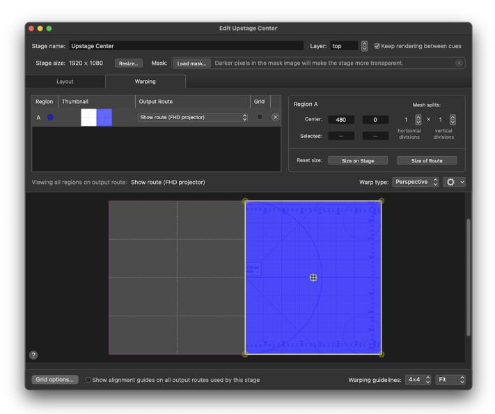
The result is that the right half of the cue is displayed using the right half of the device.
