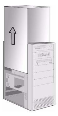
**Figure 3-9.** Removing the Workstation Cover (example)
