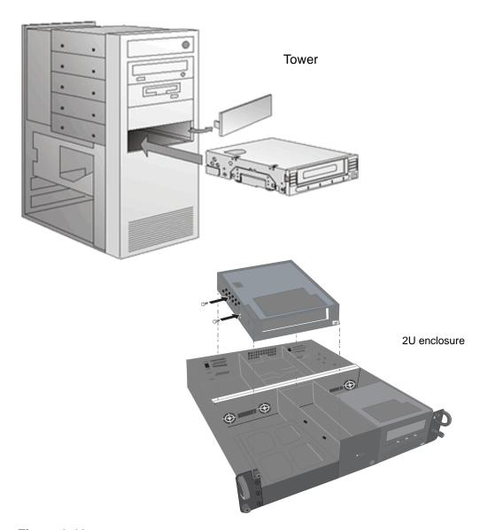
**Figure 3-10.** Tape Drive Installation in an Open Drive Bay
