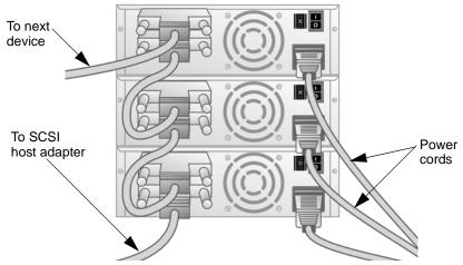
Figure 3-3. Tape Drive SCSI and Power Cable Connections
