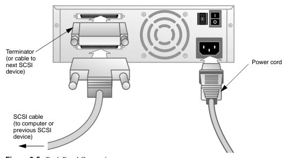
Figure 3-5. Back Panel Connections
