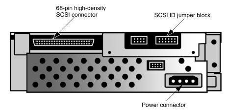
Figure 3-6. Back Panel Connections, Internal Tape Drive
