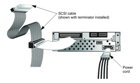
**Figure 3-11.** SCSI and Power Cable Location (Internal Tape Drive)
