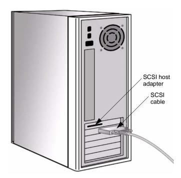
Figure 3-4. Server SCSI Cable Connections
