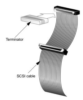
Figure 3-7. Terminator Installation
