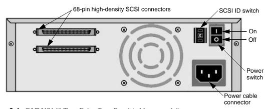
**Figure 3-1.** DLT VS160 Tape Drive Rear Panel (tabletop model)
