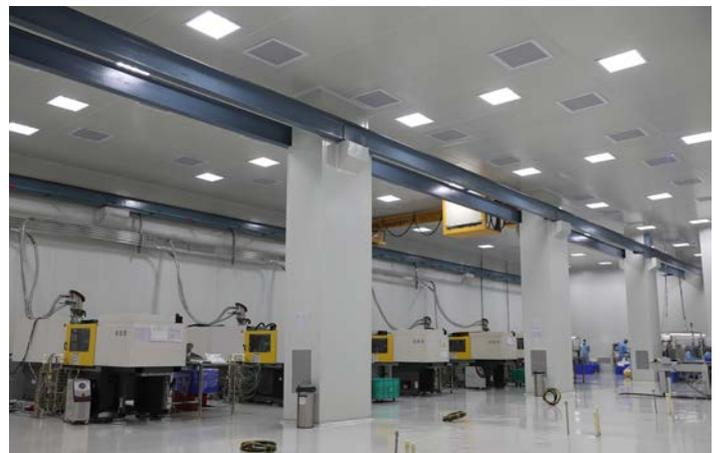
Facility validated from ISO CLASS 8 & equipped with latest robotics & automation machines
