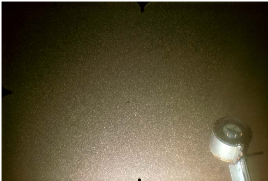
Figure 3.4.7.1. “Bed-hop” camera image taken at Lihir station L1, showing the seabed obscured by a dense haze of suspended particles. Width of image at lower edge approximately 1m, depth of field approximately 2.5 m.
