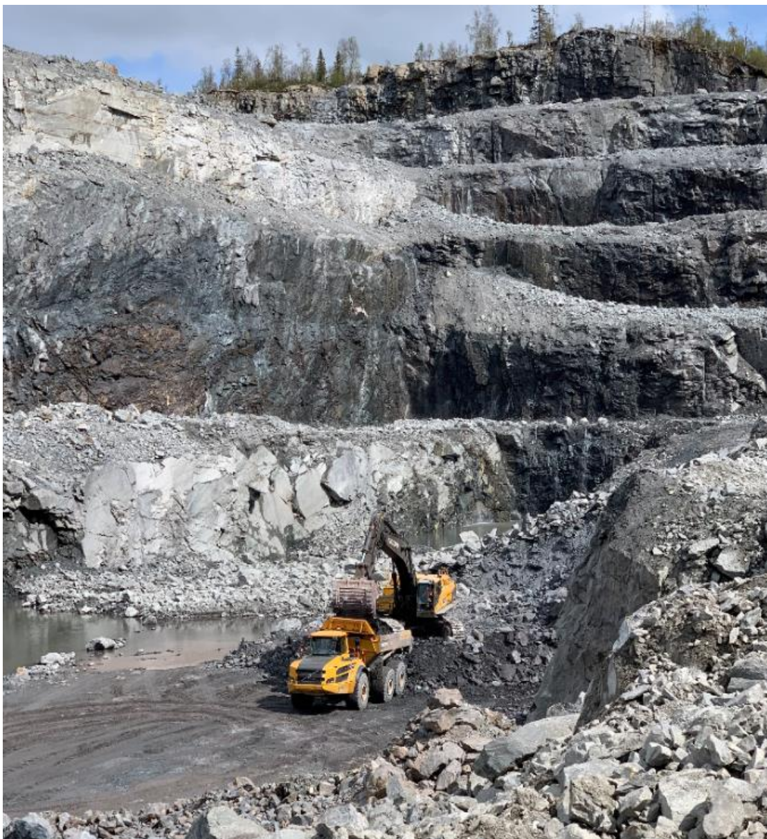
Figure 10-16: Mining in the Kvannevang open pit with the iron formation clearly visible in the pit wall (Source: BGS)
