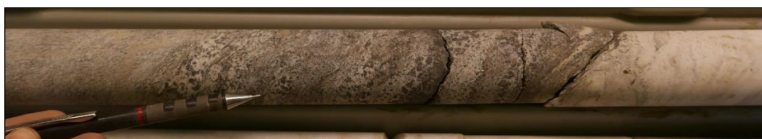
Figure 6-7: BH75-2011, 153 m, Intervals rich in Mag clusters at schist - marble contact (Source: SGM)
