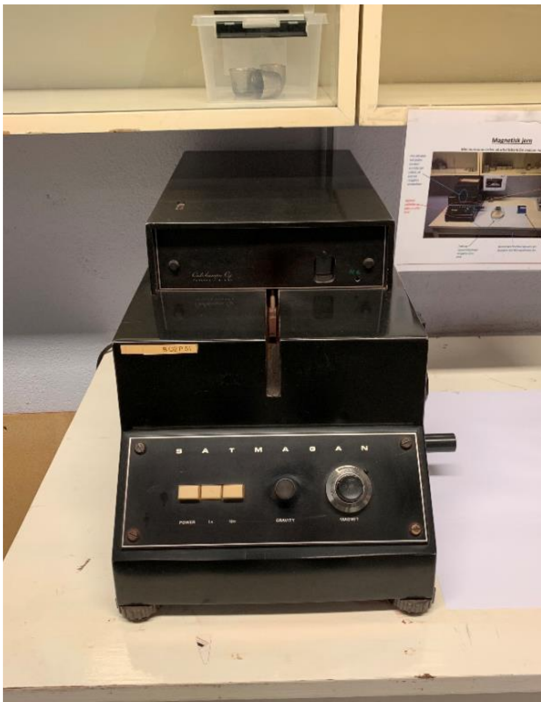
Figure 10-7: Satmagan for Fe_Mag determination (Source: BGS)
