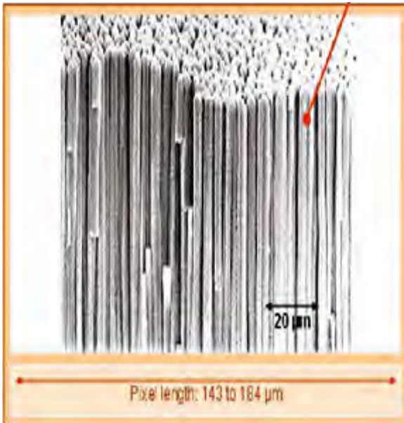
Fig. 7.54. The CsI crystals can be grown in needle-shaped form, measuring 5–10 μm. The size of one detector element (154 μm) defines (among other factors) the spatial resolution in an acquisition mode without binning (pixel binning). In order to reduce the size of data sets to be reconstructed, programs with various binning modes (1×1, 2×2 detector elements), faster rotations and fewer projections are used
