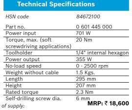
Scope of supply: Carry case; Depth stop; Magnetic universal holder; Screwdriver bit; Belt clip
