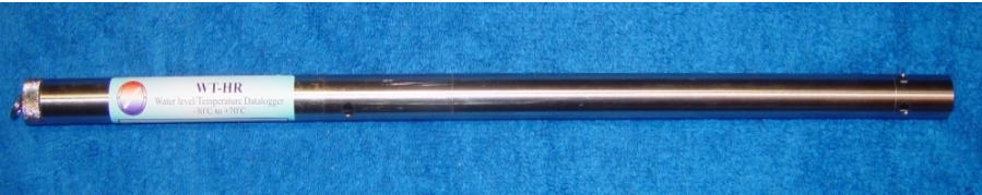
Figure 5.4: The loggers used in water table monitoring. This particular logger has a 25 cm water level sensing zone.
