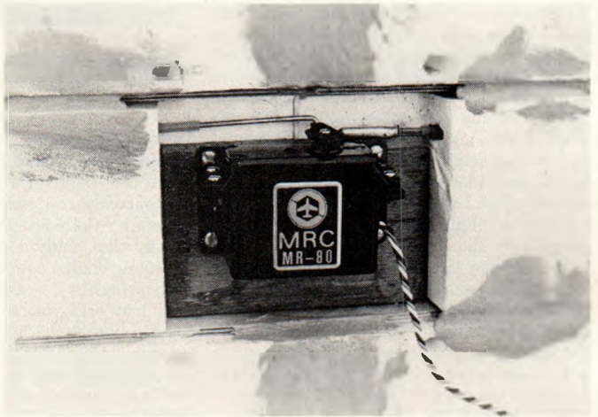
The MRC MR-80 servos used are lost in the cavernous R/C compartment (above). Receiver and battery are under the foam. The aileron servo, an MR-80 also, is located in a small compartment (below) on the under side of the wing center section. Dark splotches are filler material.
