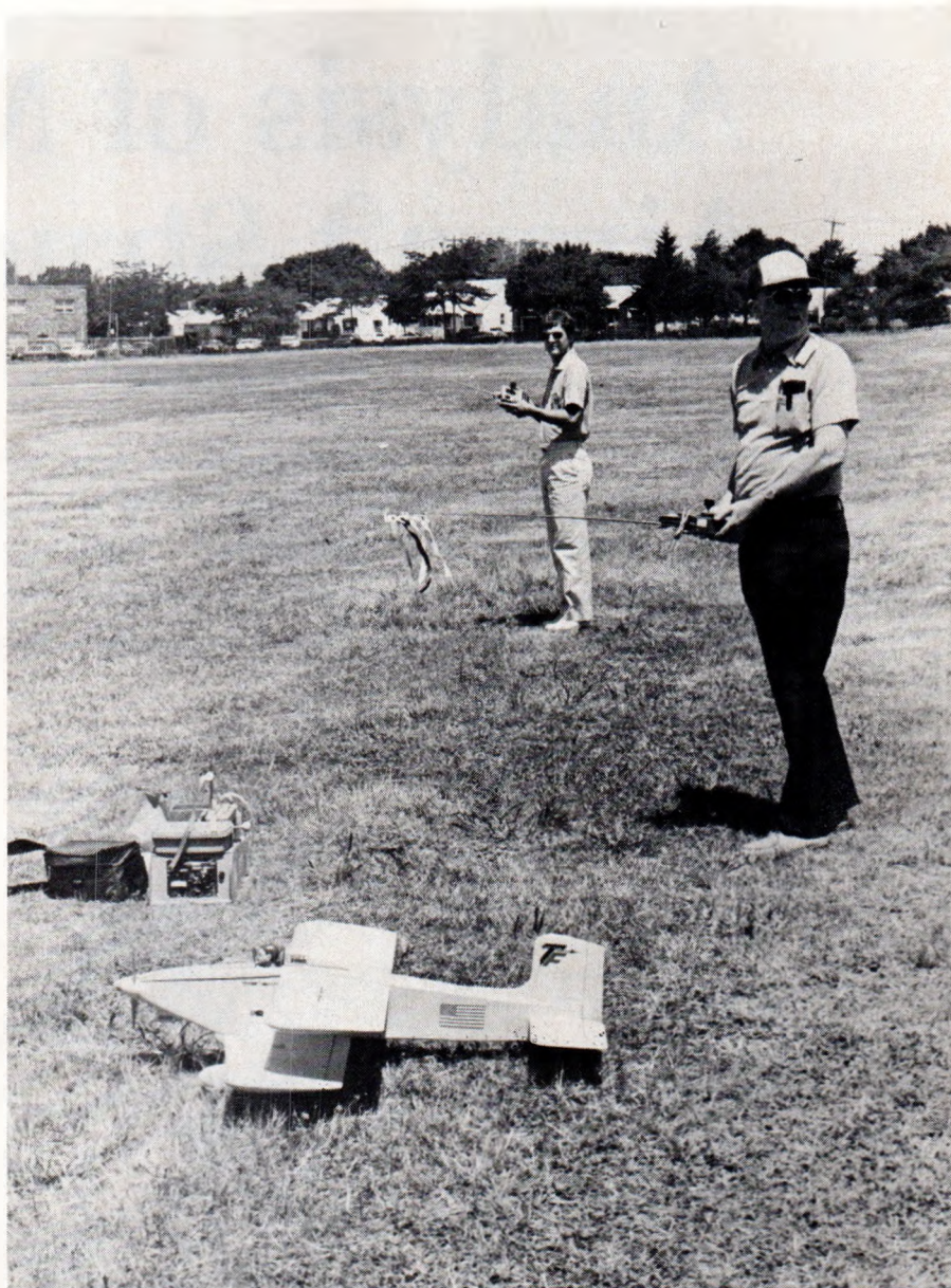
Running the all important ground interference check. In the background, Ralph Fisch holds the Airtronics transmitter exactly 30 feet away from the model. George Myers holds the interfering transmitter at just 12 feet away. Only at that distance did the 10 kHz away signal begin to cause a problem.
