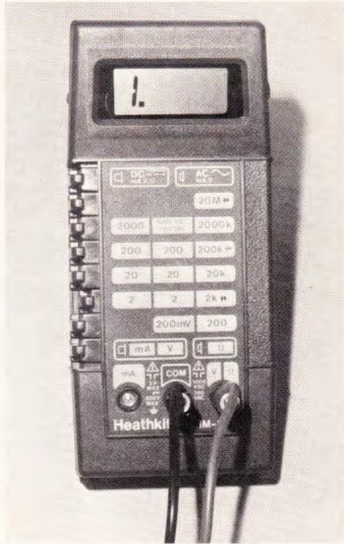
This is what you would see if you attempt to take a reading in excess of the selected scale. Unit has good overload protection. Good unit.
