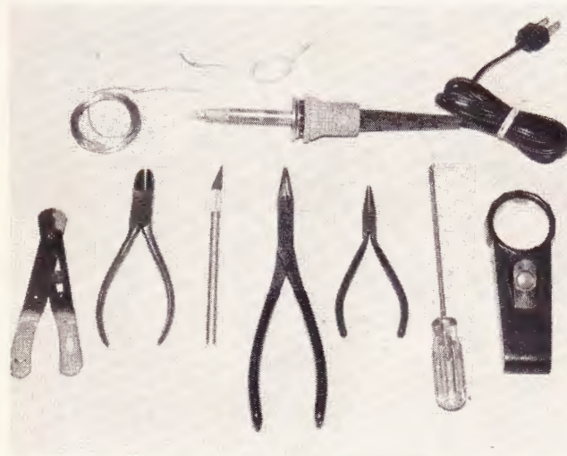
Simple assortment of tools is all that is necessary to put the Heathkit IM-2215 Digital Multimeter (above). Major components ready for final assembly (below). L.C.D. display gets soldered to the main board.
