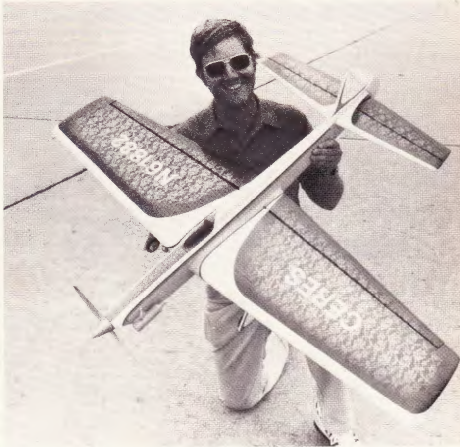
Bob McDonald assumes the "classic" pose of builder with plane (above). In this case, the plane is Bob's own design Ceres. The stylish stunter features "I" beam wing construction and elegant lines (left).
