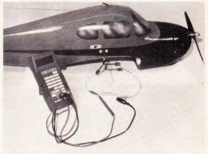
All the components assembled to the main printed circuit board (above). I.C.'s not plugged into sockets. Using the Heathkit D.M.M. with a simple load resistor for discharge test (below). Procedure outlined in August FM.
