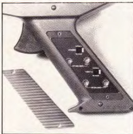
Bob Aberle shows how the MRC Grand Prix radio is used in actual operation (above). Top view of Speed Handle Control (top). Major controls visible. Inside Speed Handle Control unit (above left). Quite an assortment of electronic parts here. Additional controls found by removing one side of handle grip (left). Steering and throttle channels have reversing switches. Each of these two channels also have individual throw controls. All in all, a very versatile radio. Loaded with features.
