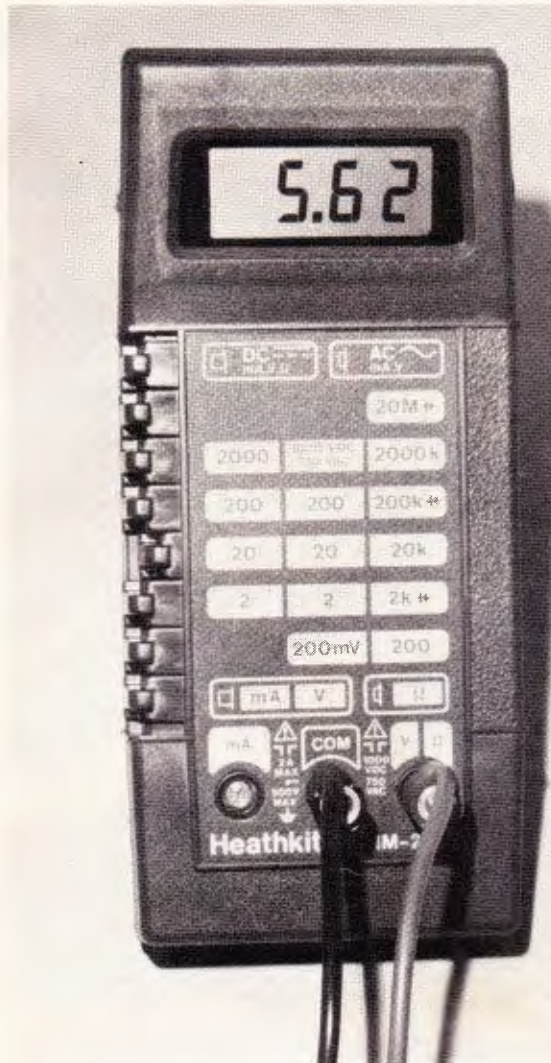
A typical reading of an airborne battery pack at roughly full charge. Numerals are 0.5 inches in height. Quite easy to read. Nice feature.
