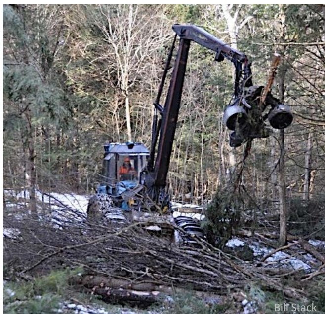
Figure 9. Manual and cut-to-length harvesting affords opportunities to enhance forest floor structure by topping and limbing at the stump. Harvests conducted by feller-buncher call for other approaches to retain debris on site.
