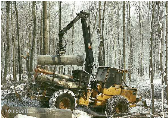
A winter selection harvest with a forwarder minimizes leaf litter and understory damage, as well as risk to nesting birds. Cleaning soil and plant parts from equipment limits the spread of invasive plants and earthworms.
