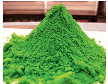
After cleaning the fraction, fluorescent powder can be reprocessed into new phosphors.
