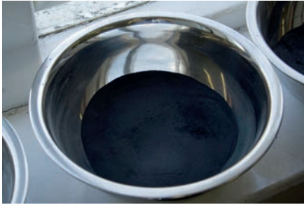
Magnetite: this magnetic material is quite heavy, especially when compared to the cenospheres. RockTron wants to develop a process to make this material suitable for use in dense media separation.
