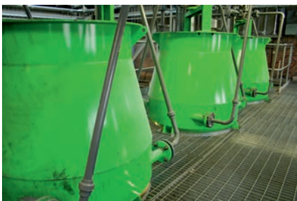
Pneumatic flotation vessels: RockTron uses three types of vessel to float the carbon.
