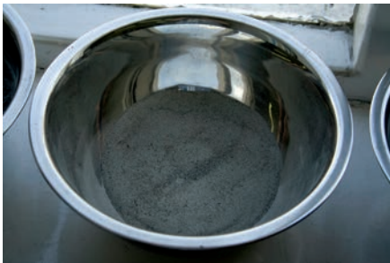
After the removal of cenospheres, carbon and magnetite, the remaining solid alumino-silicates are separated into a coarser and finer fraction: alpha and delta particles. This bowl contains delta particles.
