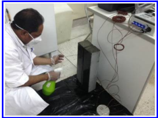
Plate 1. Application of spray coating curing.
