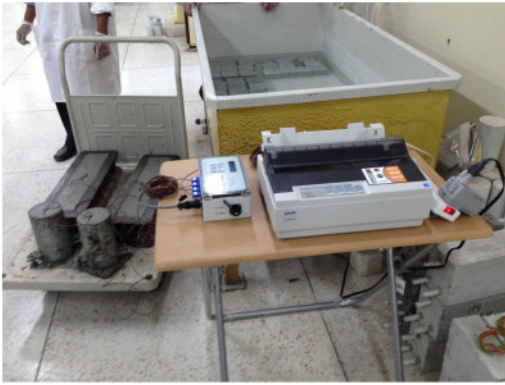
Plate 2. Connecting specimens to maturity meter.
