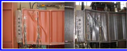
Figure 6. a) After loading of Joint 1; b) After loading of Joint 2.
