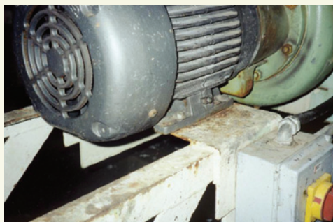
Figure 2: This motor is mounted on a piece of flat bar, which is flexing.
