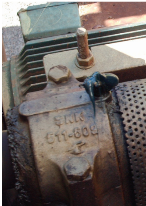
Figure 1: More bearings fail due to over greasing than under greasing
