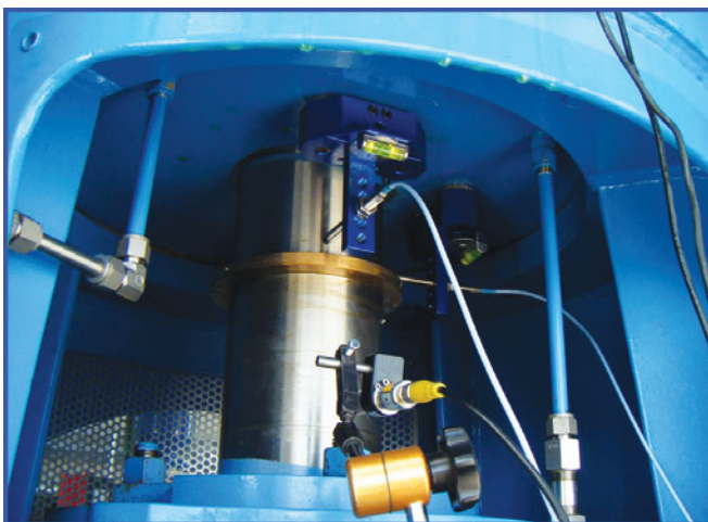
Figure 7: CMS removable probe holders mounted on vertical pump
