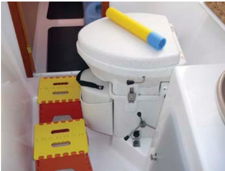
↑ The yacht has a composting toilet to eliminate plumbing and storage tanks and their associated hassles.
