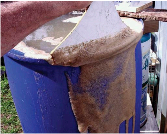
↑ It looks scary, but the foam is all of the water's contaminants being removed by the electroflocculation process.
