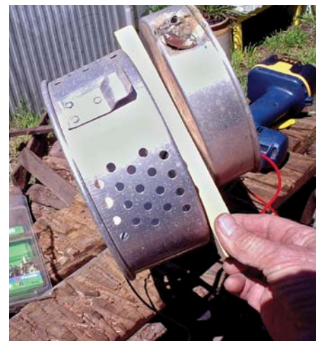
↑ The pans are screwed to either side of the insulator to act as electrodes.
