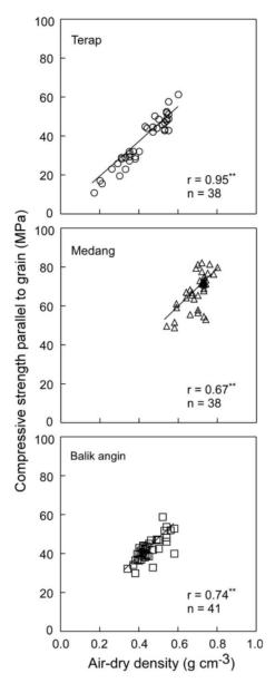
Figure 6.—Relationships between air-dry density and compressive strength parallel to grain. n = number of samples; r = correlation coefficient; \*\* = significant at the 1 percent level.
