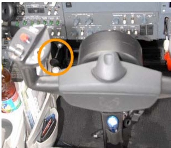
Figure 3: The actuating lever for the parking brake is located left of the commander's control column (circled in orange).
