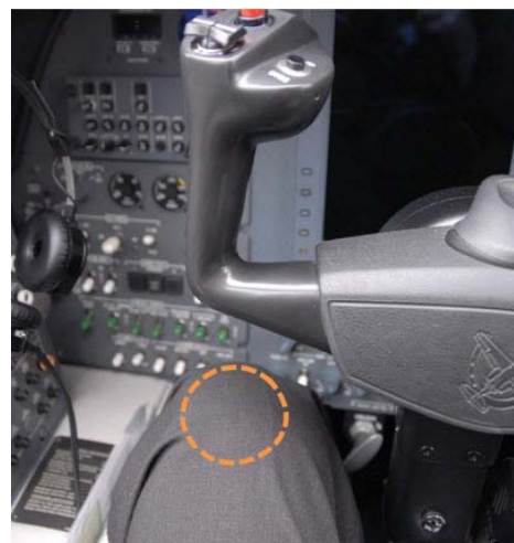
Figure 4: The actuating lever of the parking brake is concealed by the commander's left knee.
