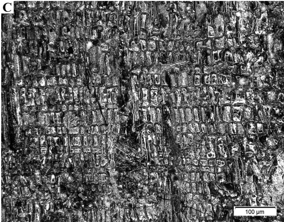
Fig. 5: A) TS: Mean tangential diameter of vessel lumina smaller than 50 \mu\text{m} . Parenchyma-like fibre bands alternating with ordinary fibres. B) TLS: Rays heterocellular, with prismatic crystals in ray cells. C) RLS: Rays with procumbent, square and upright cells mixed throughout the ray.
