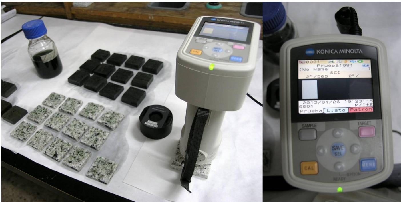
Fig. 5.4.1. Konica Minolta CM-700d Portable Spectrophotometer.
