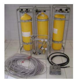
Figure 3. Set of used equipment for gas release from the sea bottom.
