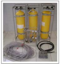
Figure 3 - Set of used equipment for gas release into the sea bottom.
