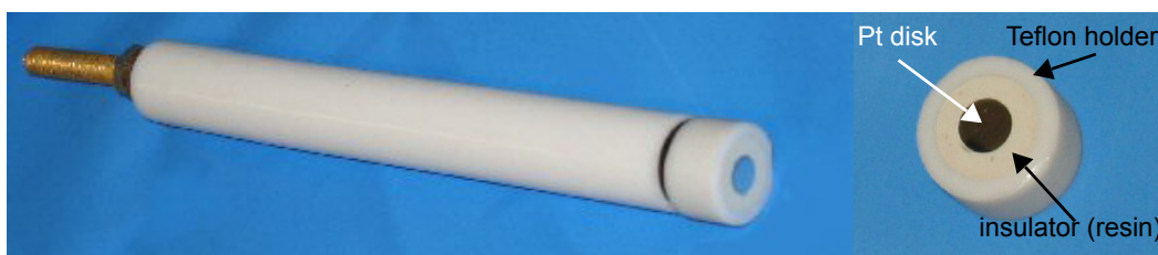
FIGURE 5.12 Photograph of Pt working electrode and electrode support.
