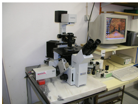
FIGURE 5.21 Photograph of the inverted microscope used in the fluorescence measurements.
