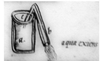
Figure 101: Illustration of the siphoning process of a bucket, F. 199r, II.91
