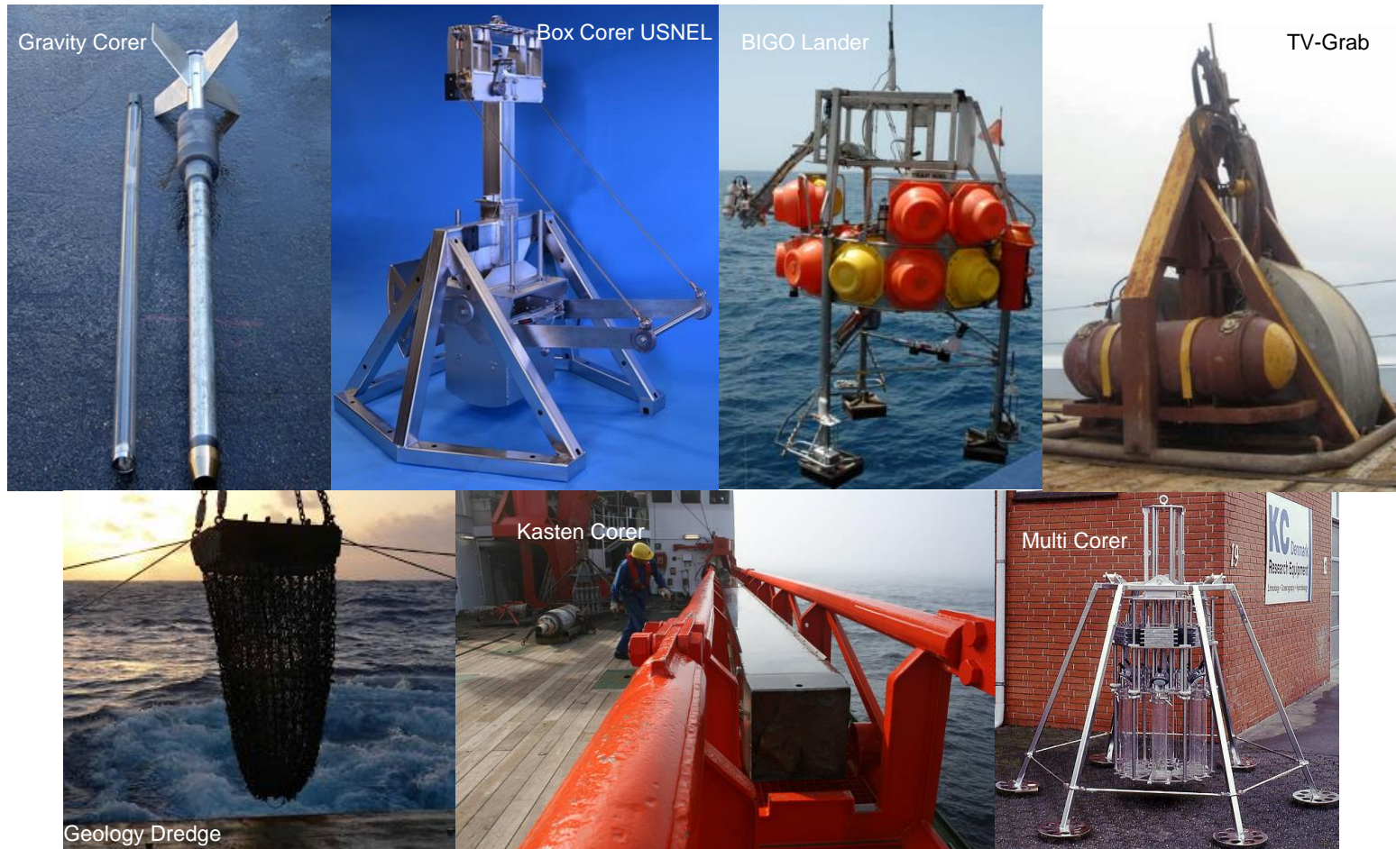
Figure 4.1 – Examples of gear used to collect the samples analysed in this work. Gravity Corer - Mooring Systems, inc. website: http://www.mooringssystems.com/ ; Box Corer - KC Denmark website: http://www.kc-denmark.dk/ ; BIGO Lander - Pfannkuche et al. , 2006; TV-Grab - Pfannkuche et al. , 2006; Geology Dredge - American Geophysical Union website: http://blogs.agu.org/ ; Kasten Corer - Alfred Wegener Institut website: www.awi.de ; Multi Corer - Alliance for Coastal Technologies website: http://www.act-us.info/ .
