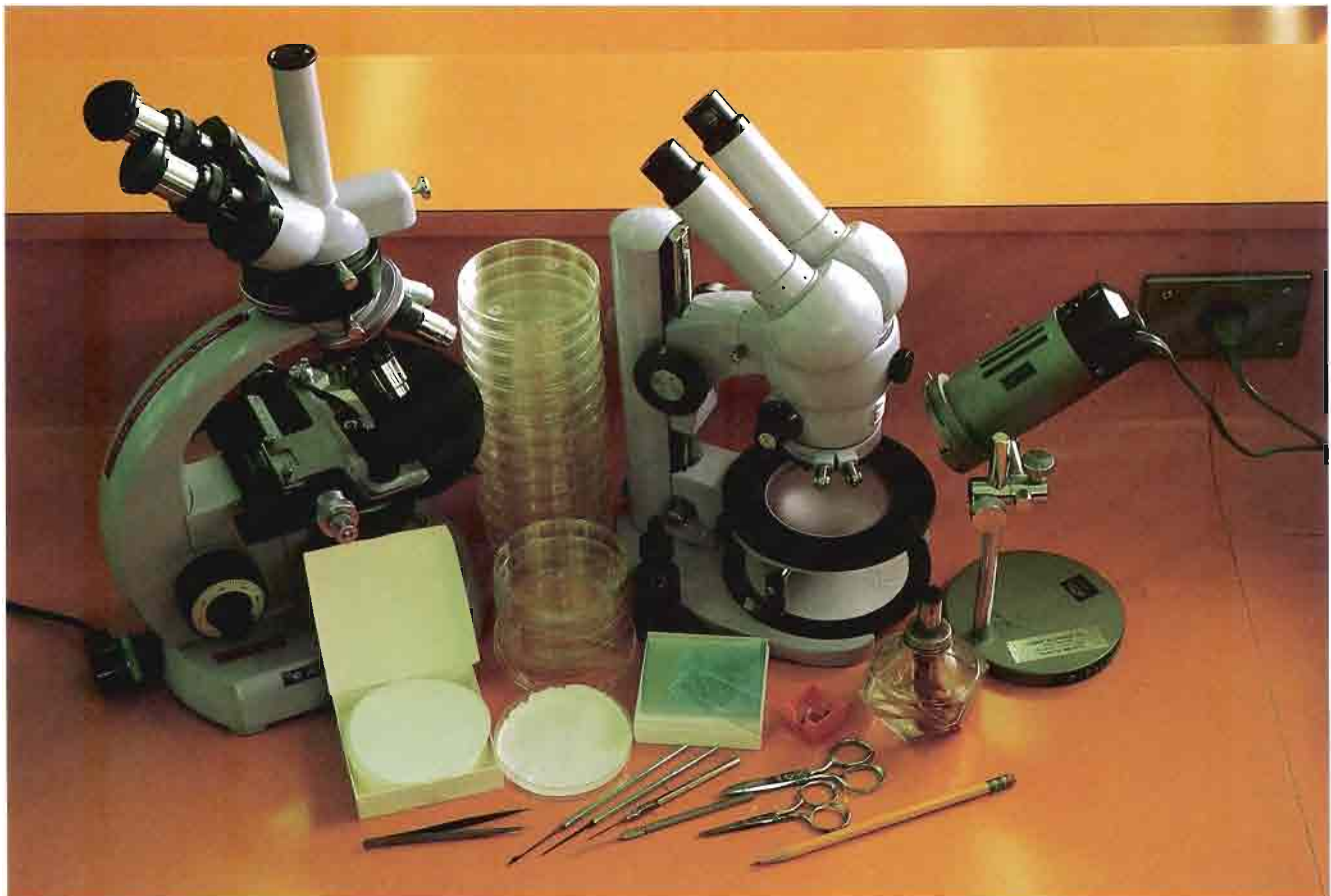
Figure 5. Equipment needed for making laboratory observations includes two kinds of microscopes (dissecting and compound types), petri dishes, filter paper, tweezers, dissecting needles and scalpel, a water dropping bottle, and glass slides with cover slips.
