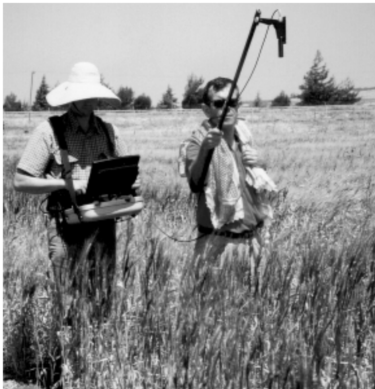
Picture 1. How to place the foreoptic while measuring radiation reflected by a wheat canopy.
