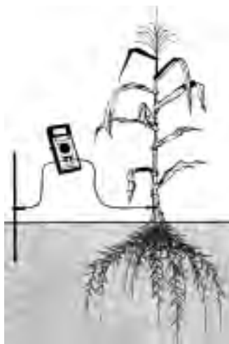
Figure 3. Electrical capacitance measurement of root size in a maize plant.
