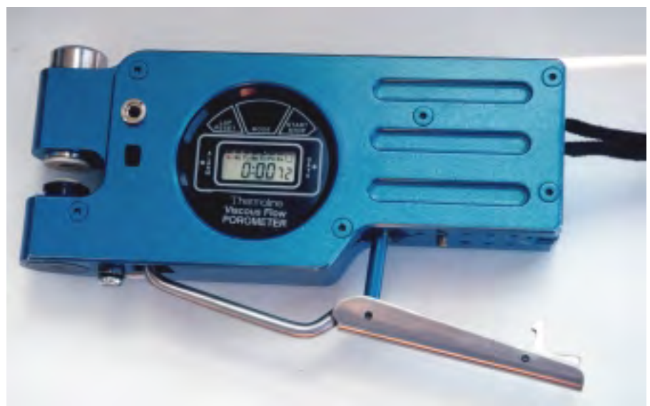
Picture 7. Viscous-flow porometer used to measure leaf stomatal conductance. It takes between 10 and 20 seconds to do single measurements on healthy wheat plants.
