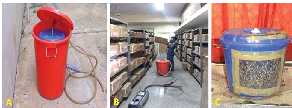
Figure 9. (A) Moth collection device; (B) moth collection using suction pump; (C) oviposition cage.
