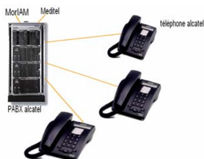
Figure II. 3 .Architecture PBX Alcatel
