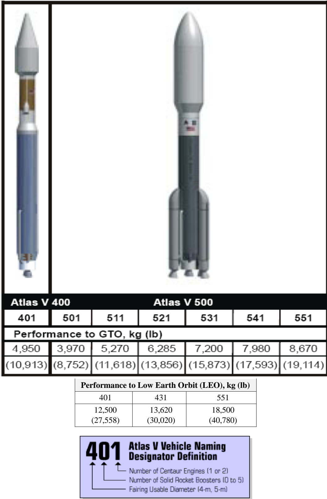
Figure 2–3. Atlas V Family of Launch Vehicles and Payload Mass that can be Lifted to Specific Orbits
