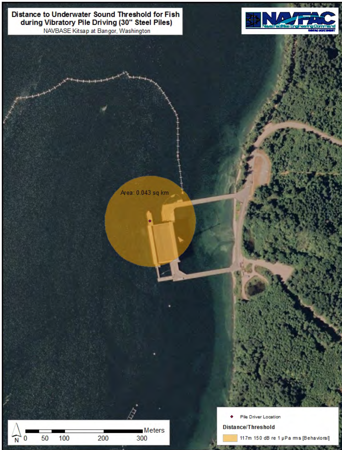
Figure 3-2. Distance to Underwater Sound Threshold for Fish during Vibratory Pile Driving (30-inch steel piles)
