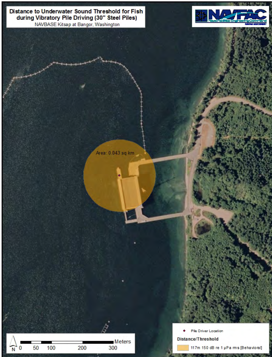
Figure 5-2. Area Exceeding Fish Behavioral Guidance Depicted for a Representative Vibratory Driven Pile.
