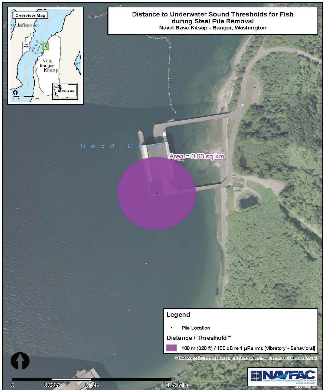
Figure 3-13 Distance to NMFS Underwater Noise Threshold from Vibratory Pile Driving During Steel Pile Removal
