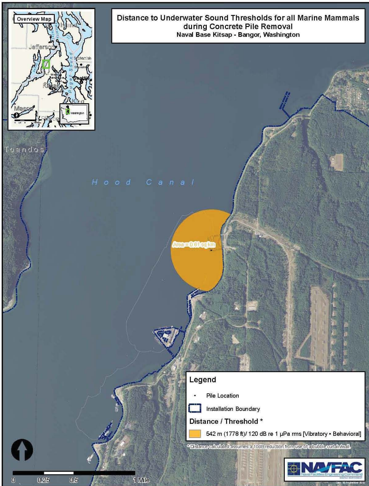
Figure 3-18 Distance(s) (m) to NMFS Underwater Sound Thresholds for all Marine Mammals from a Chipping Hammer During Concrete Removal
