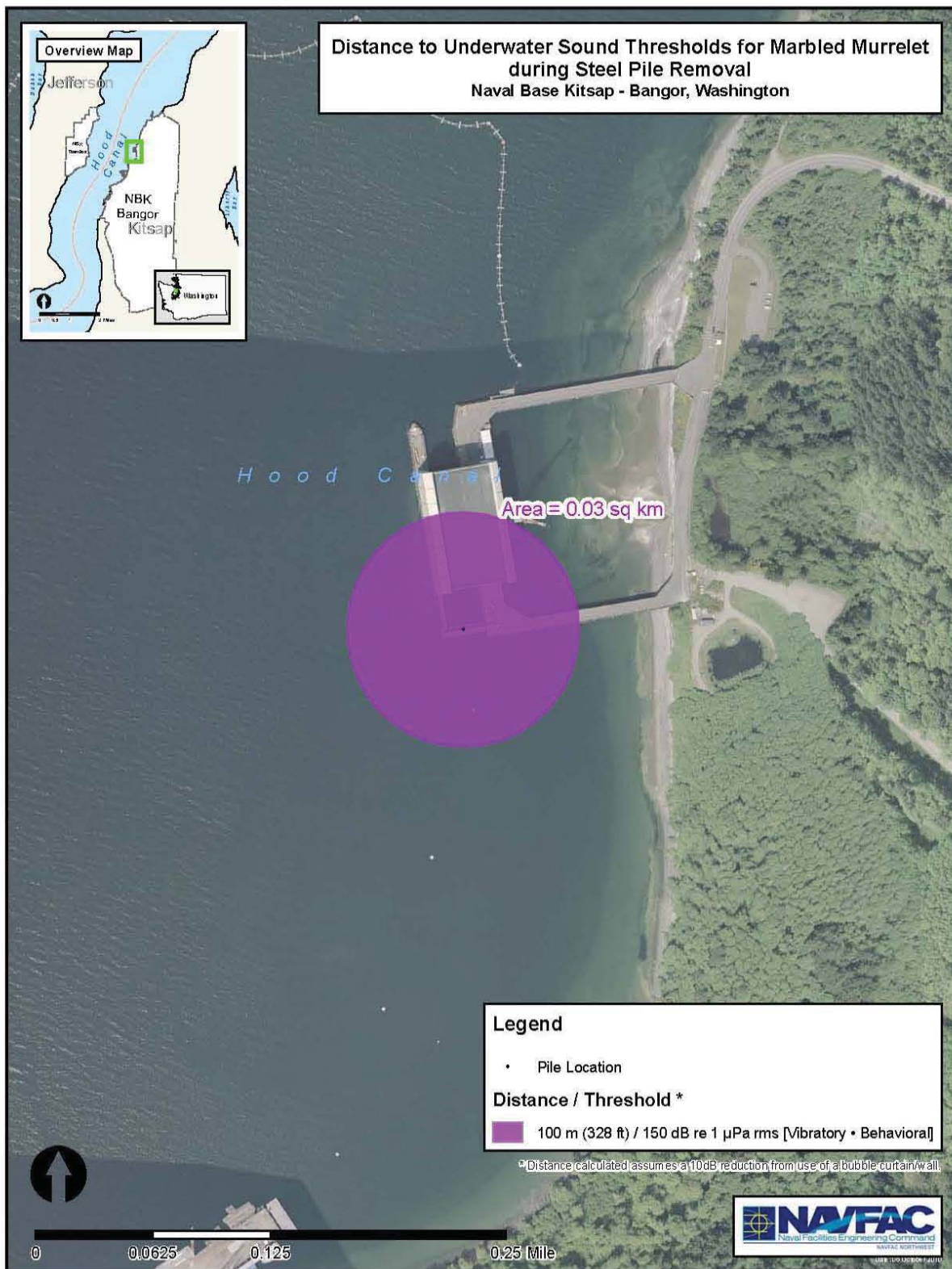
Figure 3-26 Distance(s) to USFWS Underwater Noise Thresholds for Marbled Murrelets from Vibratory Pile Driving During Steel Pile Removal
