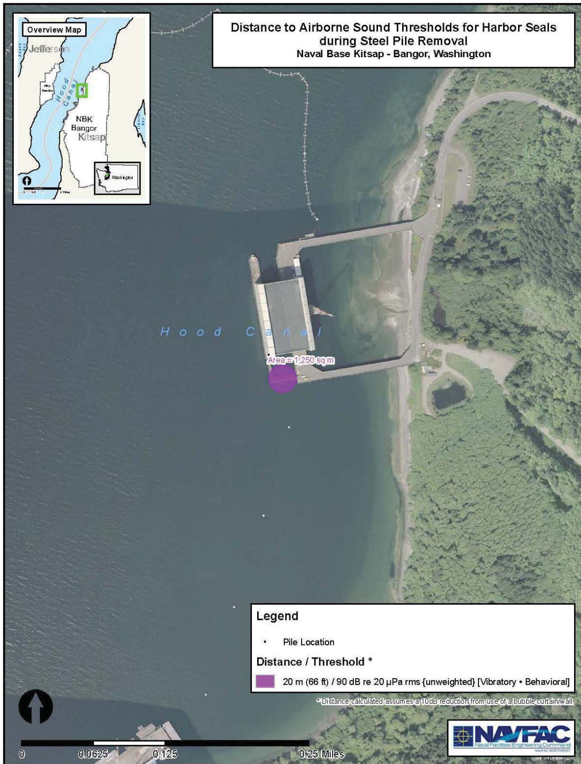
Figure 3-22 Distance(s) (m) to NMFS Airborne Sound Thresholds for Harbor Seals from Vibratory Pile Driving During Steel Pile Removal
