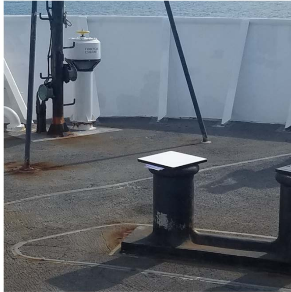
Figure 56. NOAA 'white' 99% reflectance plaque on a mooring bollard of the Okeanos Explorer foredeck
