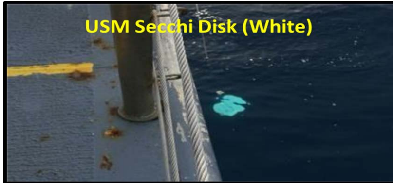
Figure 20. USM white Secchi Disk being lowered into the water.
