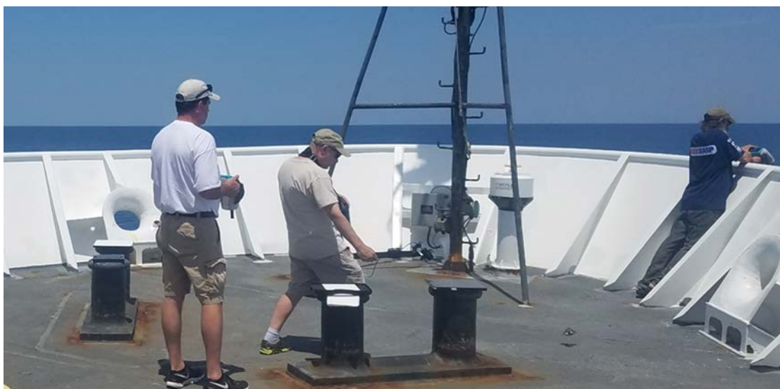
Figure 23. Example ASD shooting the NOAA grey plaque and ASD shooting the water surface for water leaving radiance.
