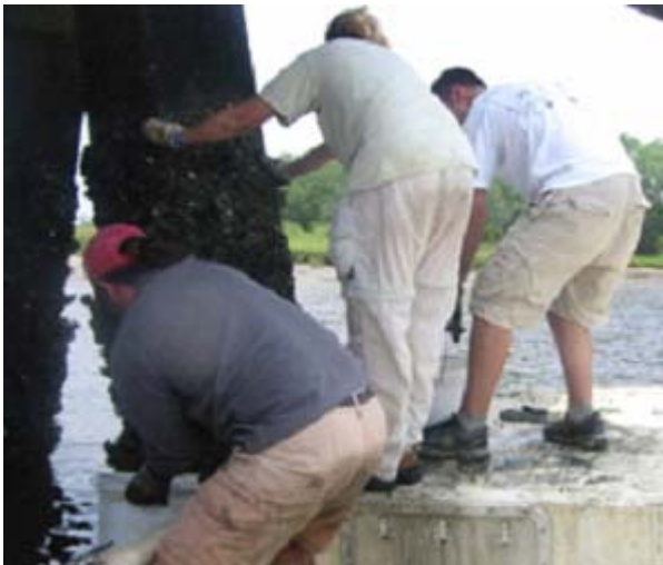
Figure 41 Taking piling scraping sample
