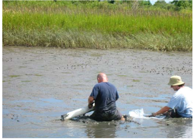
Figure 37 Taking core samples
