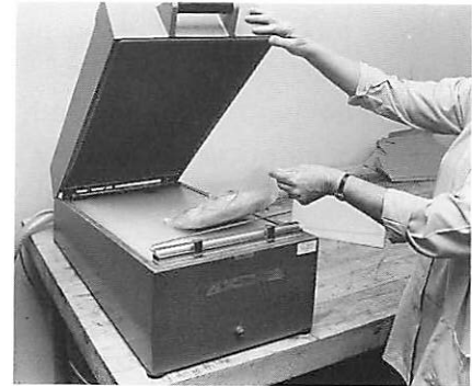
Figure 19. Open and reseal bag to achieve good air removal
