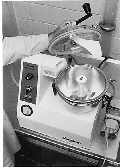
Figure 6. Vacuum cutter-mixer with 5-liter bowl
