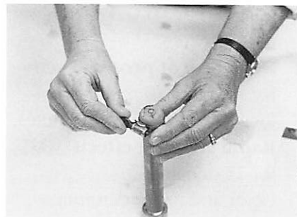
Figure 26. Clamp the rubber stopper to prevent popping off during cooking as the paste expands (if tubes are to be fully immersed in water)
