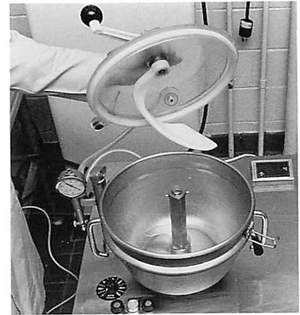
Figure 7. Vacuum cutter-mixer with 12-liter bowl
