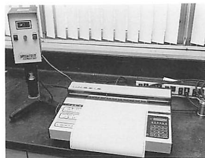
Figure 39. The torsion gelometer device with data feed to a strip chart or small computer
