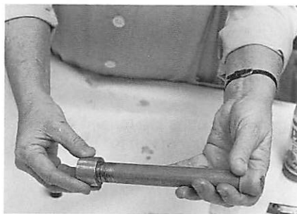
Figure 25. For stainless steel tubes, a rubber stopper is placed on one end and the other sealed with a screw cap
