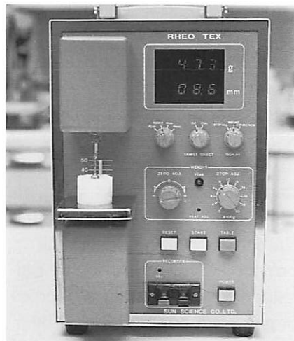
Figure 54. Electronic punch test machine
