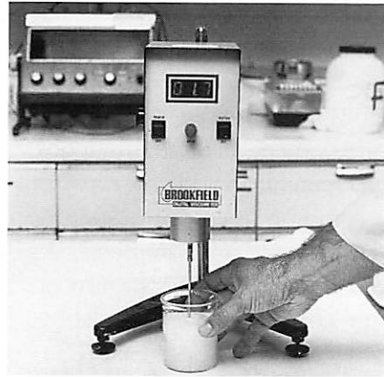
Figure 48. Measurement of the apparent viscosity of dilute solutions of surimi to estimate quality of the surimi
