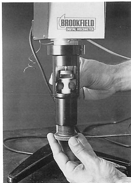
Figure 38. The milled sample is mounted into the torsion device
