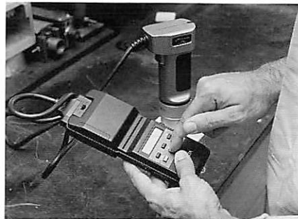
Figure 45. Enter the color coordinates of the Hitch tile into the memory of the colorimeter
