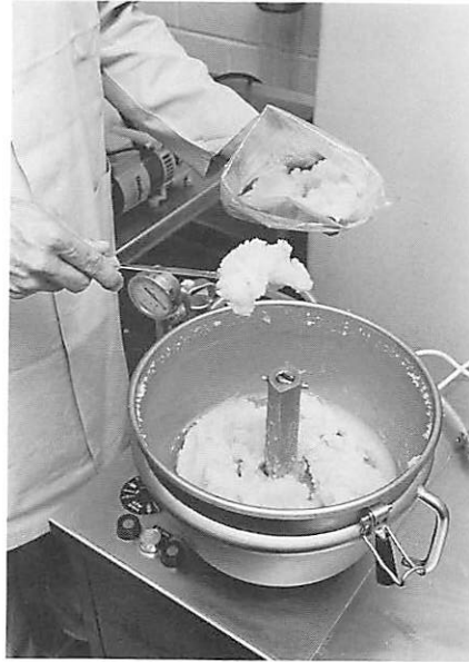
Figure 17. Loading plastic bag with chopped surimi paste for air removal
