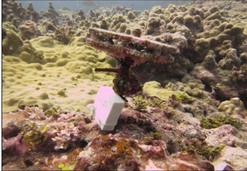
Figure A-23 Bioerosion monitoring block with CAU unit
