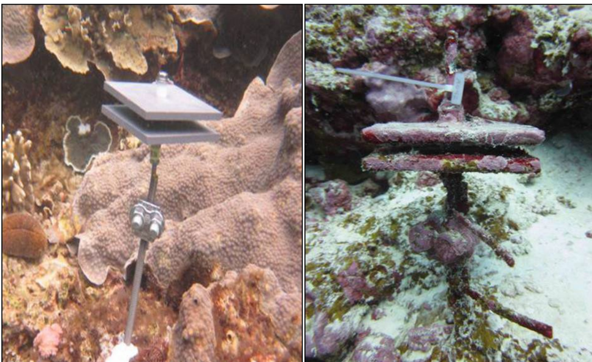
Figure A-21 Calcium acidification unit pre-deployment and two years after deployment
