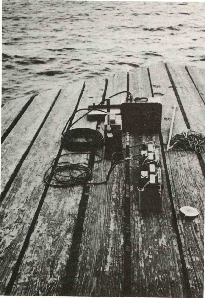
Figure 1.--Del Norte navigation system.
