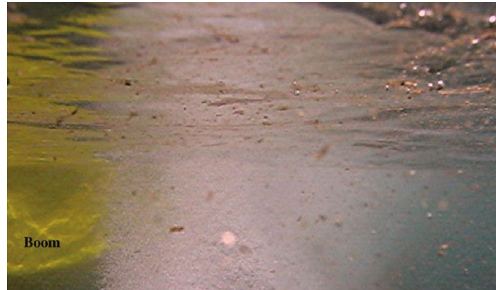
FIGURE 24: Image of submerged (dispersed) oil in the Coal Oil Point seep field during a bubble oil boom test, described in McClimans et al. [238]. Foreground oil emulsion globules are a few millimeters across. Photo is red contrast-enhanced to highlight oil. Photo: Ira Leifer.
