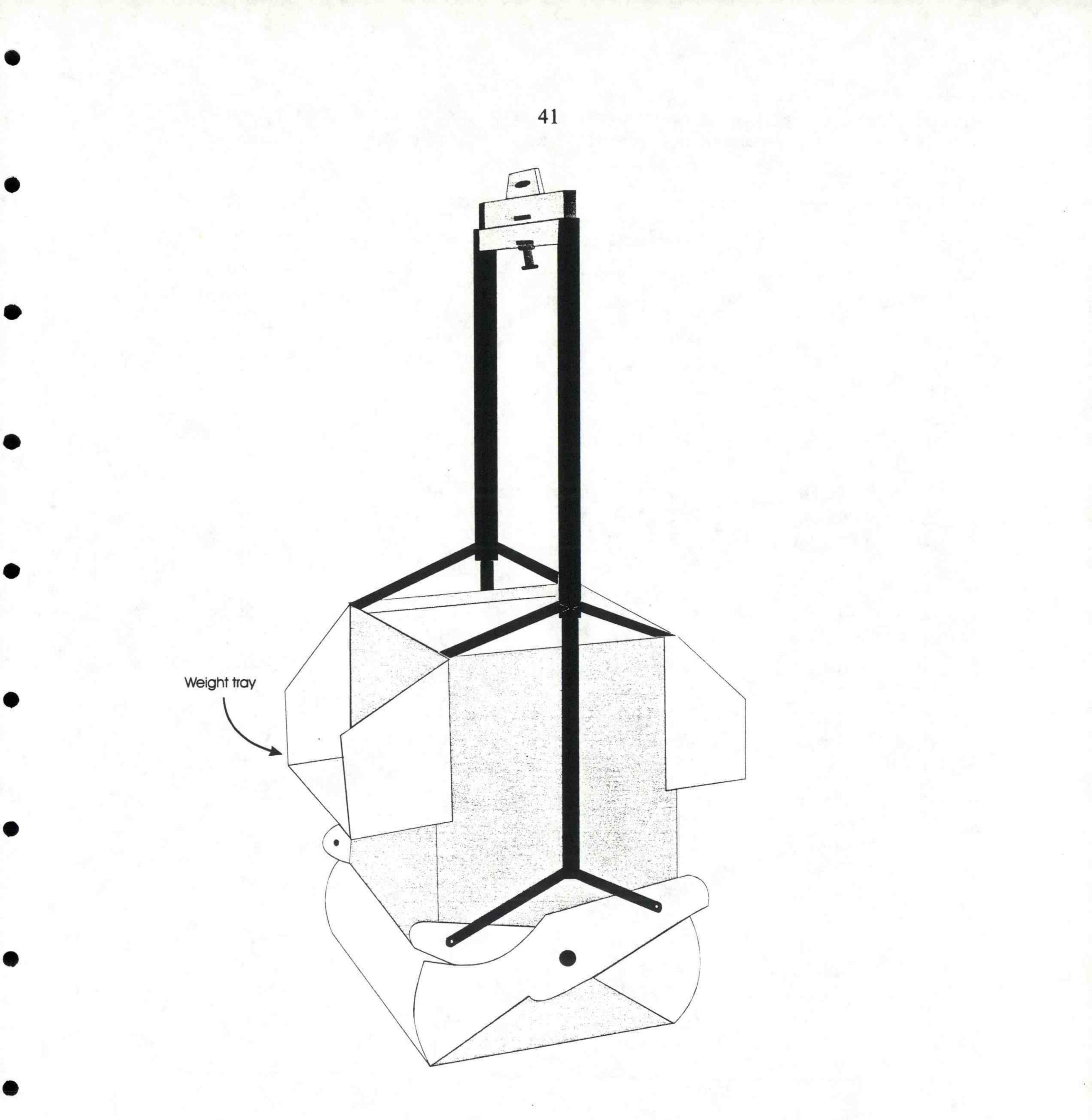
Appendix Figure 1. The 0.1-m<sup>2</sup> box corer (Gray-O'Hara modification of a standard box corer) used for benthic invertebrate sampling offshore from the Columbia River July 1993. For deeper penetration, 113-kg (250-lb) weights were placed in each tray located on opposite sides of the sampler.
