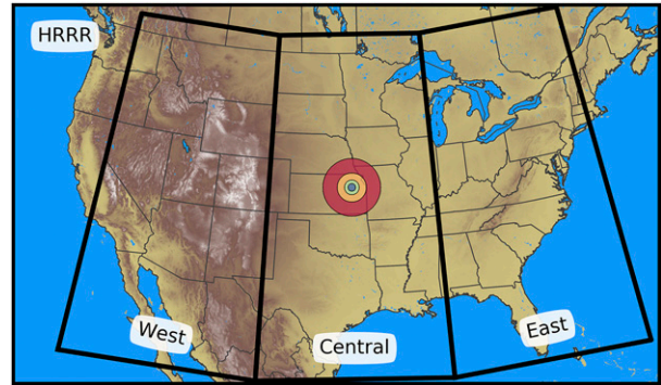
FIG. 2. The HRRR model domain, shaded by topography, with boundaries of west, central, and east subregions. Center circles represent footprints used in FSS calculations with a radius of 30, 60, 120, and 240 km.
