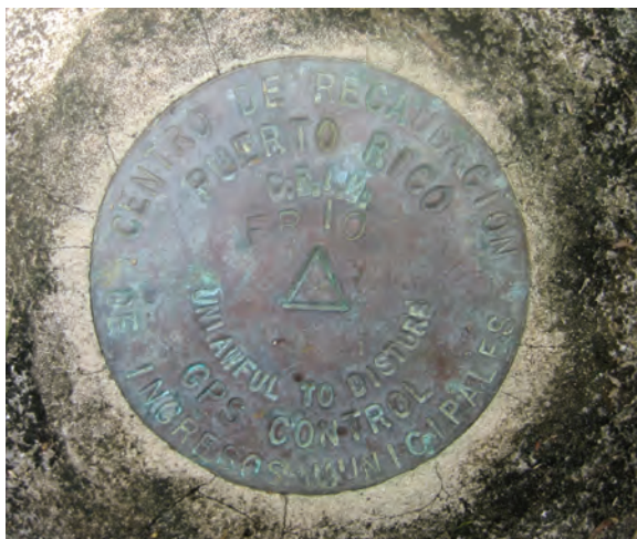
Figure 2.32. Geodetic marker from NOAA's National Geodetic Survey that was used as a ground control point.
