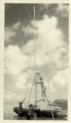
**Figure 2.** Collecting vibracore 16 off the west coast of Twin Cays with the aid of a Zodiac (inflatable boat).
