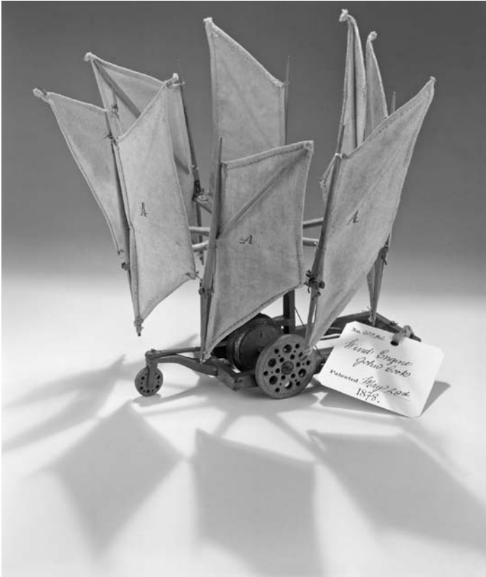
Patent No. 209,862. John Cook. Wind Engine. November 12, 1878. (SI neg. 86-6165)
