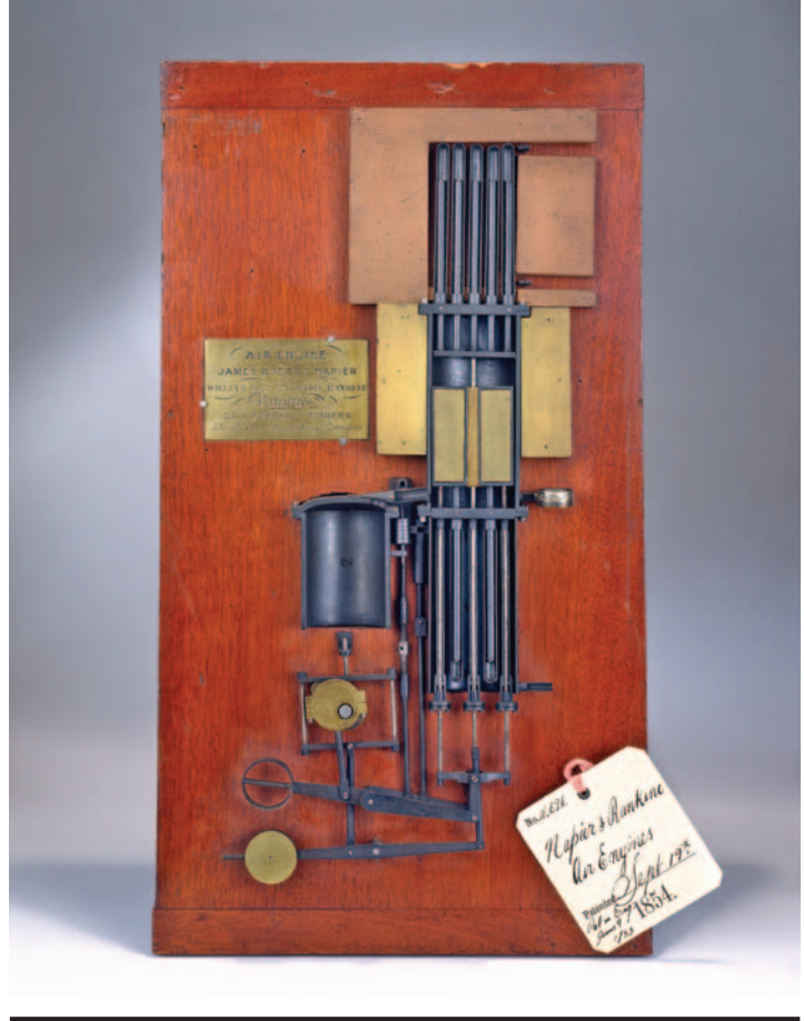
Patent No. 11,696. James R. Napier and William Rankine. Hot Air Engine. September 19, 1854. (SI neg. 86-6552)
