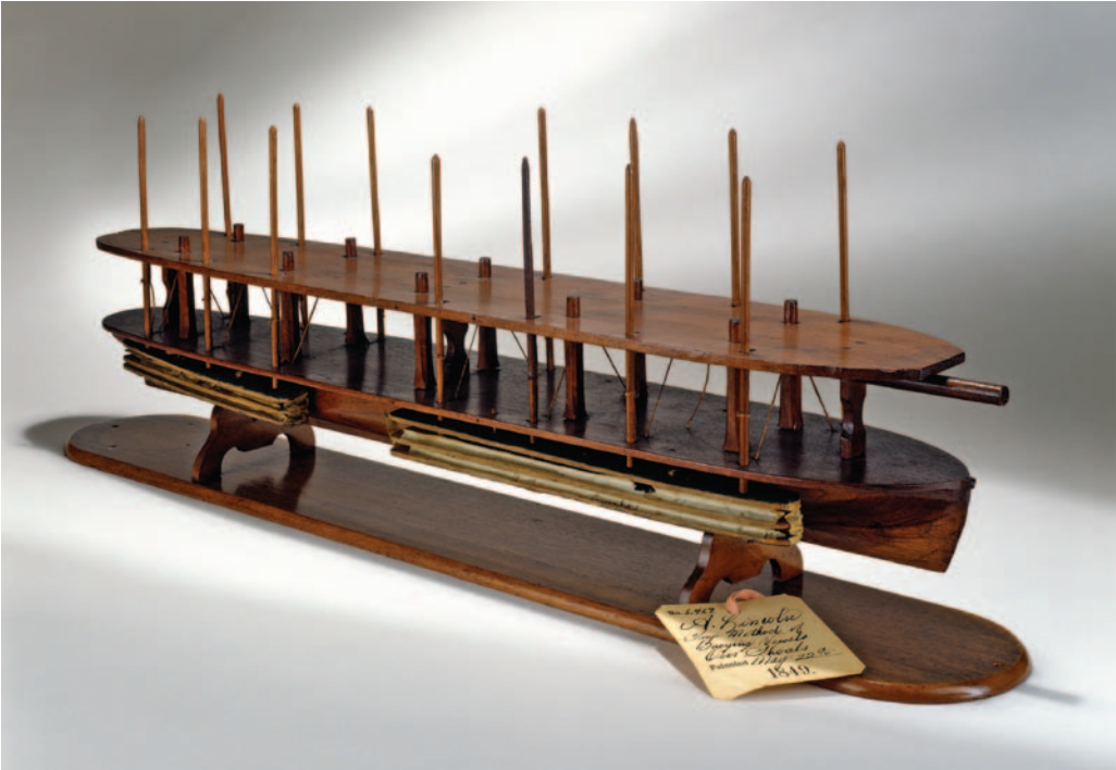
Patent No. 6,469. Abraham Lincoln. Buoyant Air Chambers for Vessels. May 22, 1849. (SI neg. 86-6162)
