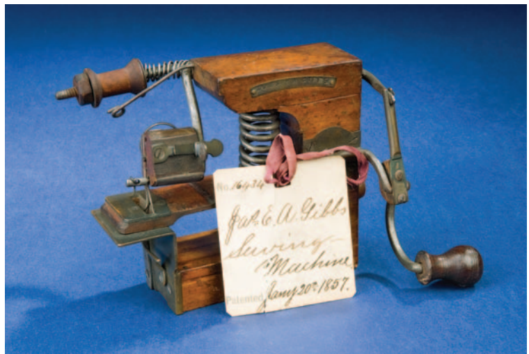
Patent No. 16,434. James E. A. Gibbs. Sewing Machine. January 20, 1857. (SI neg. 2007-6308)
