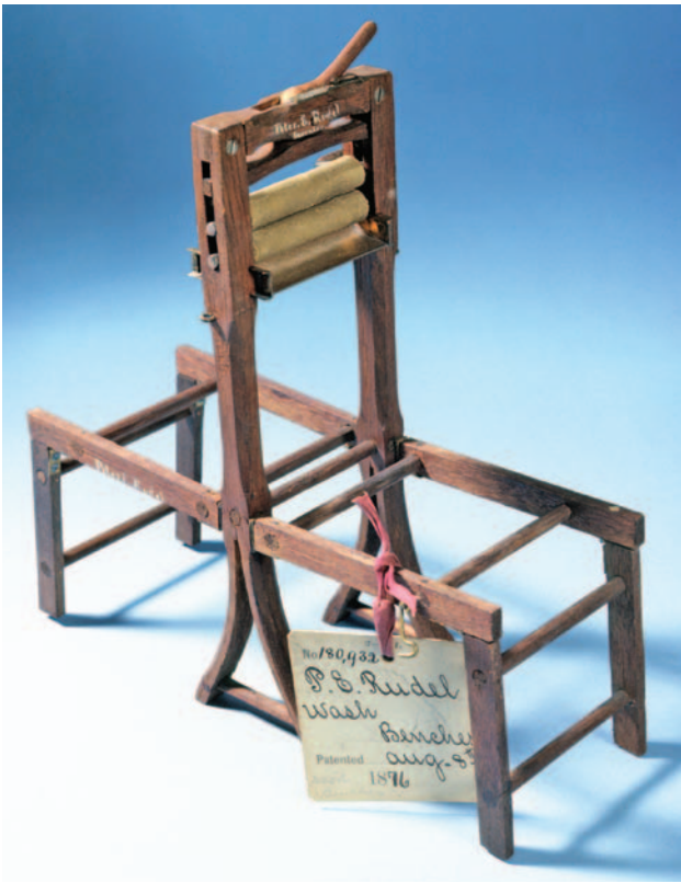
Patent No. 180,932. Peter E. Rudel. Wash Bench and Wringer. August 8, 1876. (SI neg. 80-13968)
