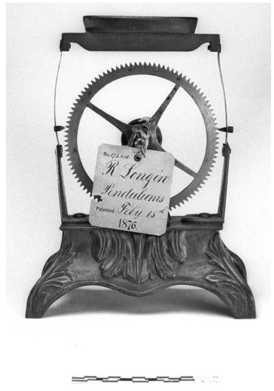
Patent No. 173,410. Raymond Longin. Pendulum. February 15, 1876. (SI neg. 83-16183.26A)
