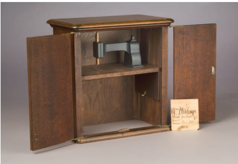
Patent No. 22,464 (detail). Doors are open showing the sewing machine still lowered. (SI neg. 2006-1877)
