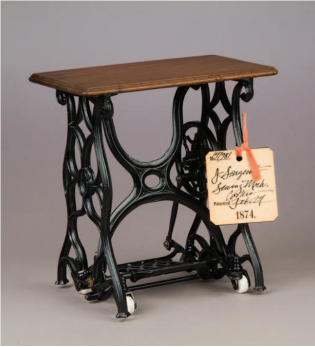
Patent No. 147,981. Joseph B. Sargent. Sewing Machine Table Casters. February 24, 1874. (SI neg. 2006-1886)
