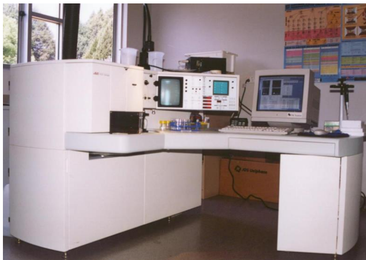
Figure 76. Flow cytometer model FACS Vantage (source: CSIRO F.D. McMaster Laboratory, Chiswick NSW).
